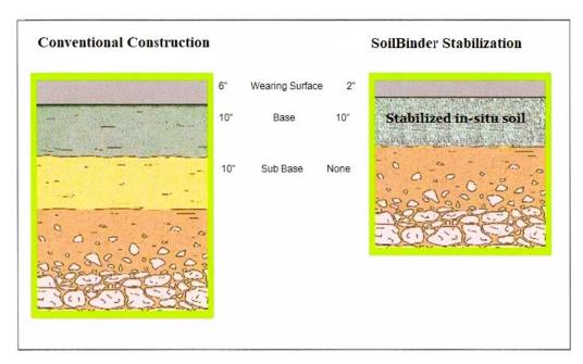
Fig. 1: Soil Stabilization using SoilBinder® vs Conventional Soil Stabilization methods.
